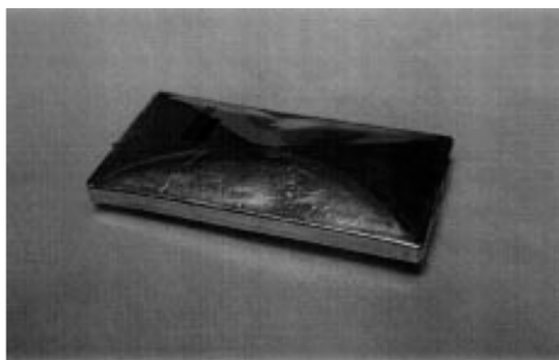
Fig. 11. Swollen shape of battery just after 1C/2V overcharge ARC test.
